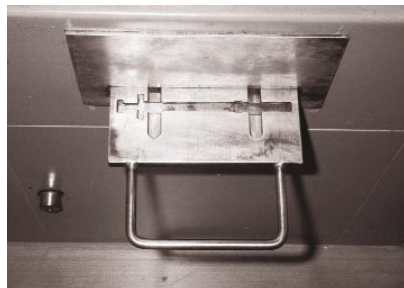
Insertion of used syringe in dispensing unit causes a new one to be released. Saxerriet Prison, Switzerland
